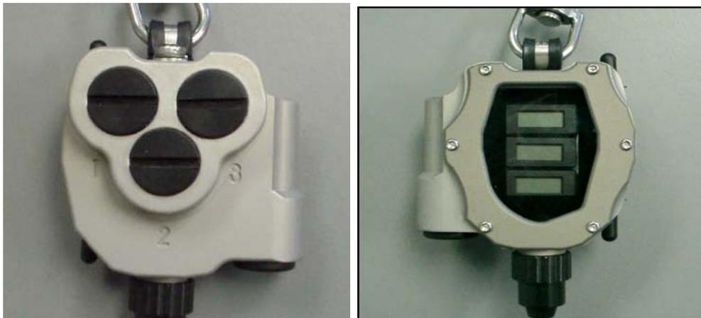
The backup display has 3 PPO2 readouts which read 3 individual sensors, an independent battery compartment, and 3 calibration potentiometers, one for each sensor.
