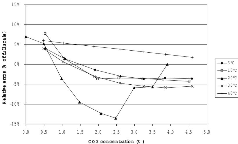
**Figure 3. Valtronics CO<sub>2</sub> sensor (Mod. 2015); temperature effects in dry gas. Relative errors (expressed as per cent of full scale) vs. CO<sub>2</sub> concentrations. Each solid line represents one temperature.**
