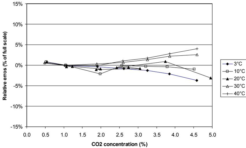
**Figure 2. Texas Instruments CO<sub>2</sub> sensor (TI9GS-4); temperature effects in dry gas. Relative errors (expressed as per cent of full scale) vs. CO<sub>2</sub> concentrations. Each solid line represents one temperature.**
