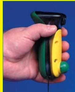
Hold the O2EII™ in your left hand, press the button once to switch on. Auto switch off after 10 minutes
