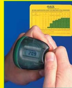
Adjust the calibration knob until the display reads the correct value, using the O2 compensation chart
