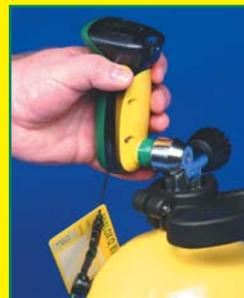
Hold the O2EII™ in your left hand and press the sample dome firmly against the cylinder outlet
